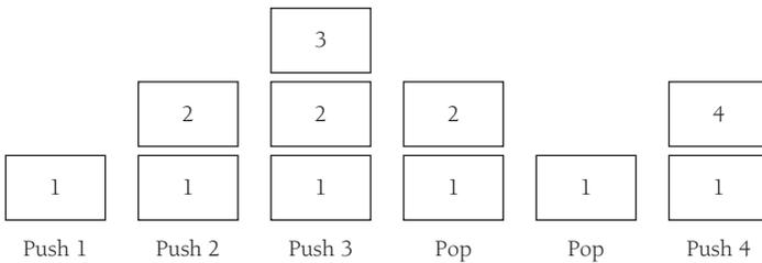
**FIGURE 5.1. Pushing and Popping a Stack.**
