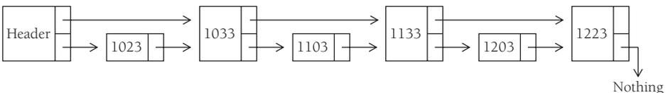
**FIGURE 15.11. Skip list with links 2 nodes ahead (level 1).**
