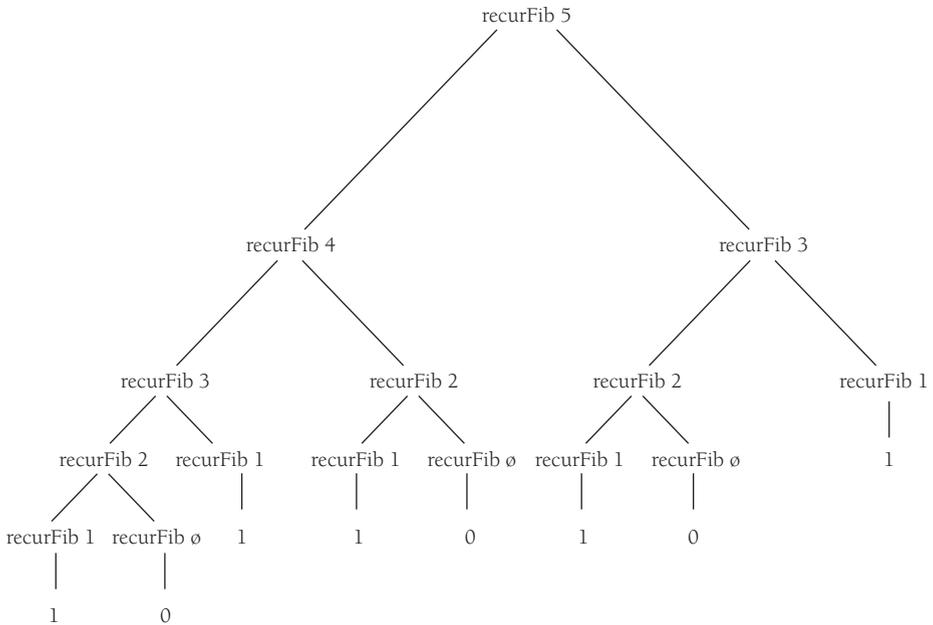
**FIGURE 17.1. Tree generated from Recursive Fibonacci Computation.**
